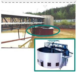
Polyus' technical team identified a possibility to boost throughput of the thickener by increasing the diameter of the feedwell
