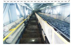
At Mill-4, the installation of an additional conveyor to transport pebble to the large cone crusher bypassing the first stage pebble crusher. This initiative allowed to avoid a decrease in productivity during the first stage cone crusher downtimes and to stabilize the ore feed preparation process
