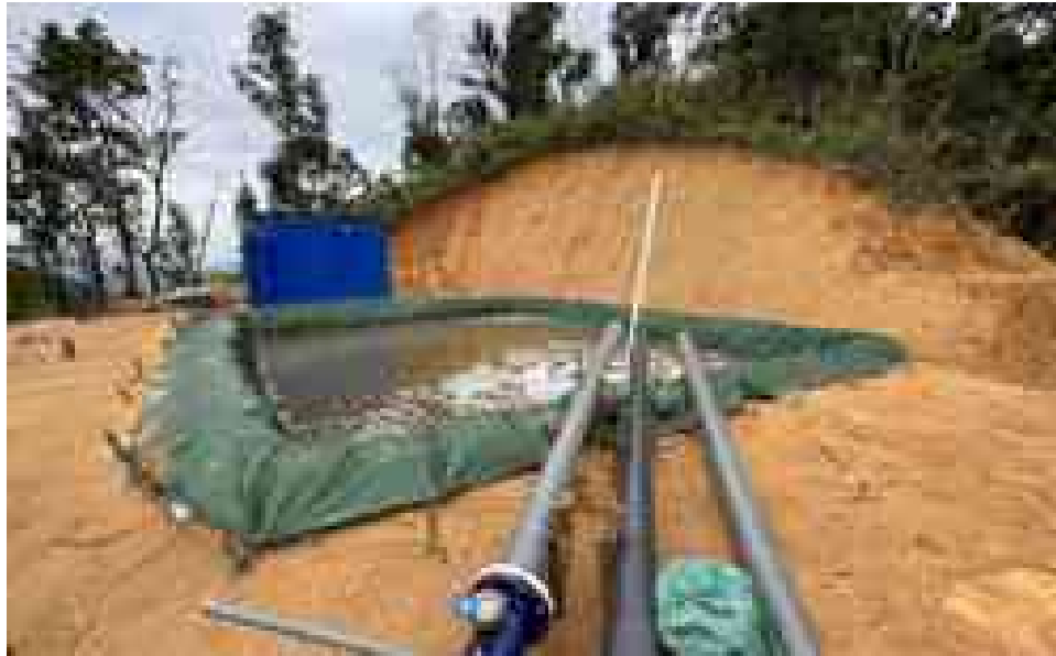
Figure 12-5: Leaching Solution Pond
