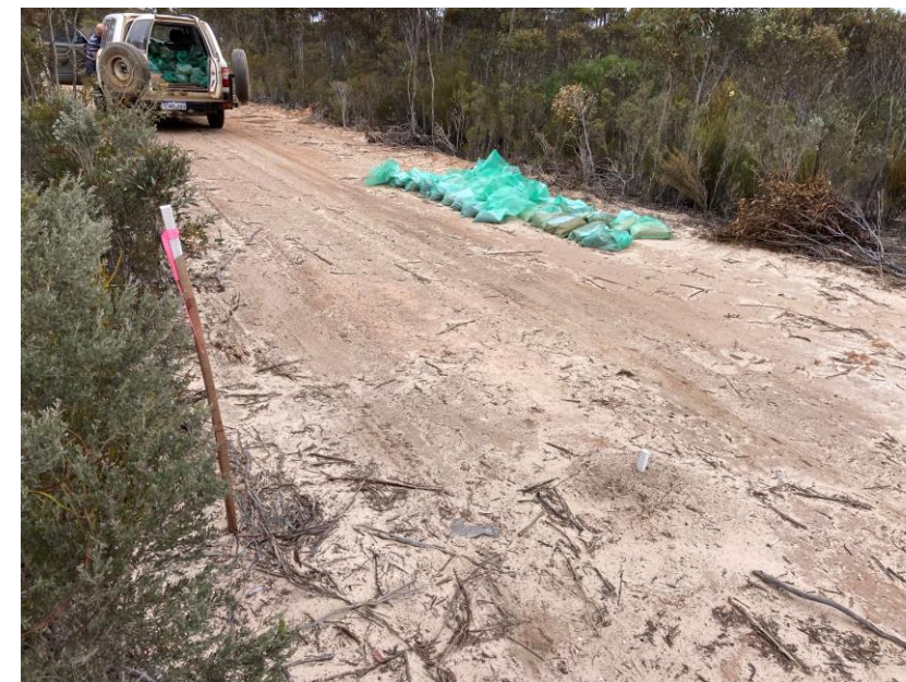
AC28 drill site at Cowalinya. Drilled by HRE in July 2021. AC28 assayed 27 metres @ 951 ppm TREO from 12 metres.
